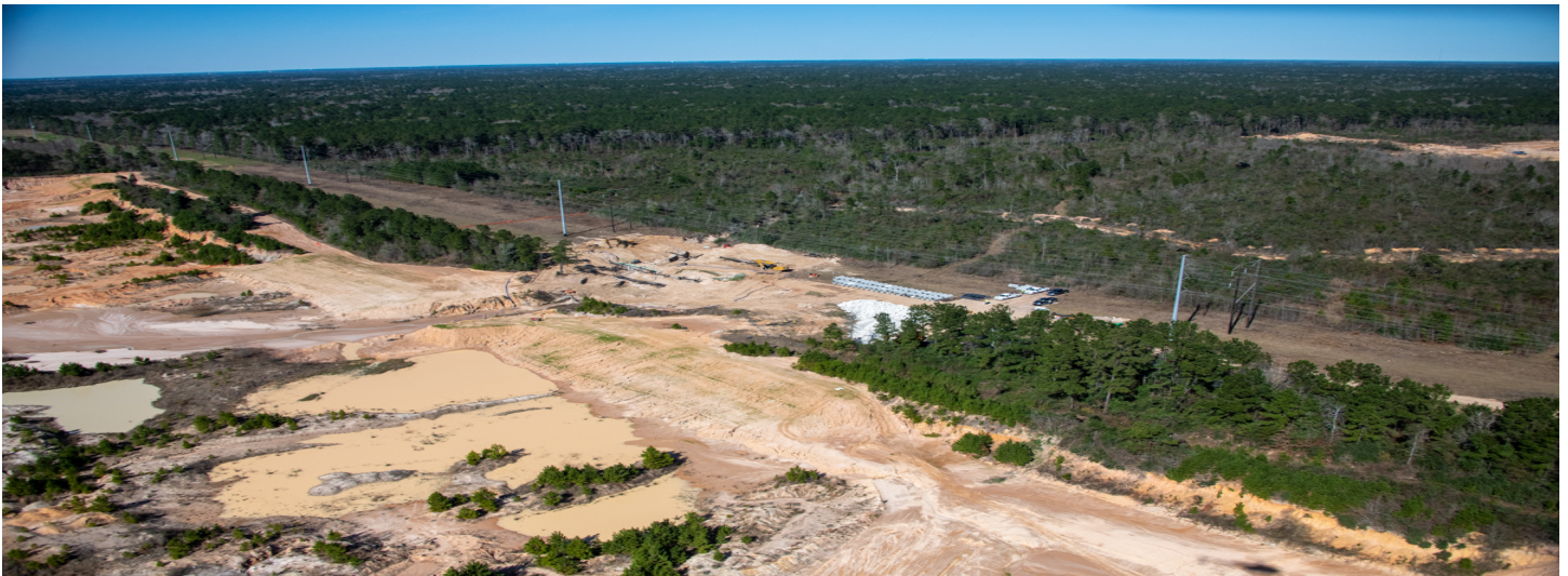
Liberty Materials undercut five pipelines carrying highly volatile liquids by mining too close to both sides of the utility corridor and then trying to drain wetlands.
